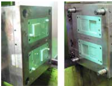
Figure 8 : PolyJet mold inserts on the molding machine. Left is the core and right is the cavity.
