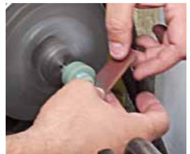
Figure 11: Finishing process of mold component.
