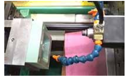
Figure 14: Cooling fixture mounted on the mold. As the mold opens, pressurized air is applied to the surface for a predetermined time.
